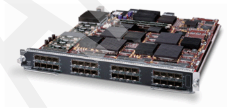
Figure 7-13 Storage Services Module
