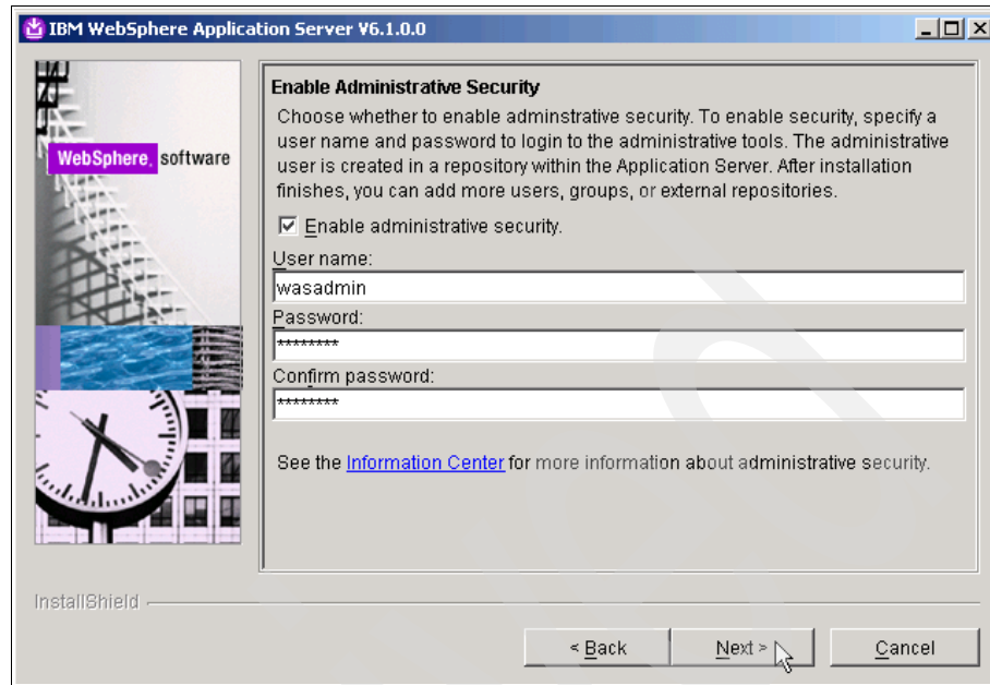
Figure 5-11 Enable Administrative Security window
