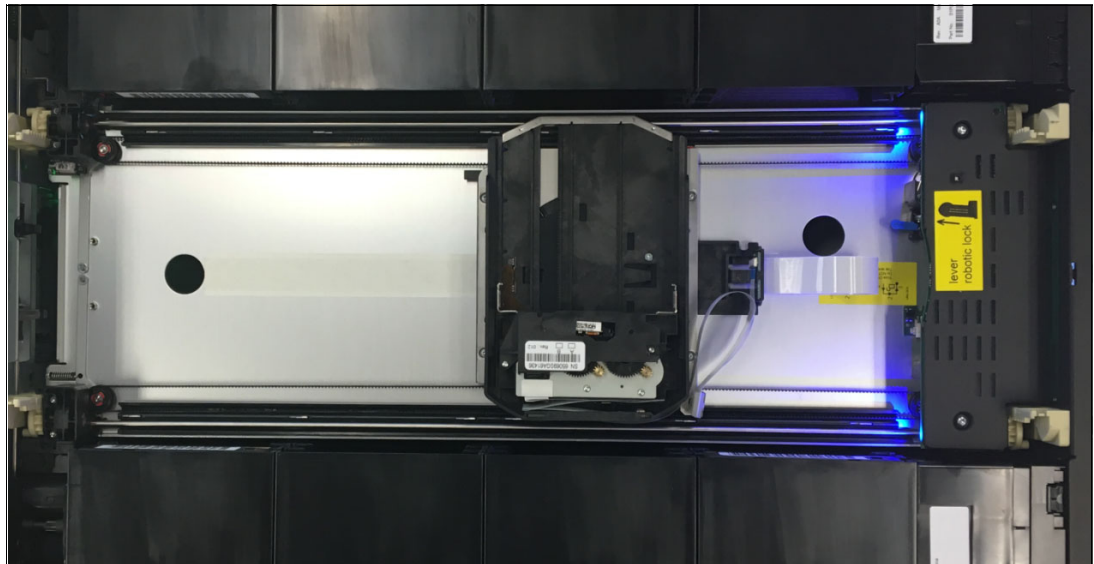
Figure 10-10 TS4300 robotic accessor
