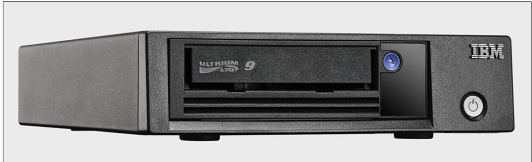
Figure 2-22 TS2290 LTO Ultrium 9 tape drive
