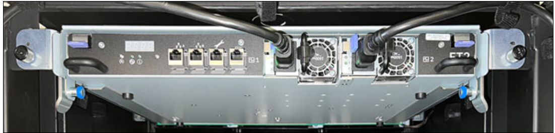
Figure 12-4 IBM Diamondback electronics tray close up
