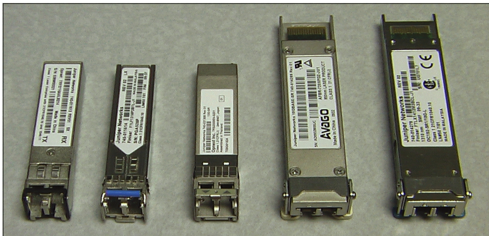
Figure 7-14 From left to right: SFP-MMF, SFP-SMF, SFP+-MMF, XFP-MMF, and XFP-SMF
