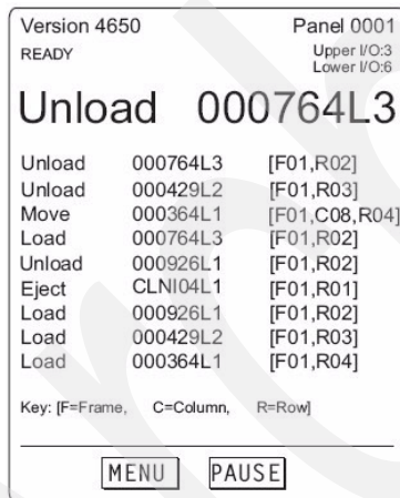
Figure 6-1 Operator panel on the 3584 Tape Library
